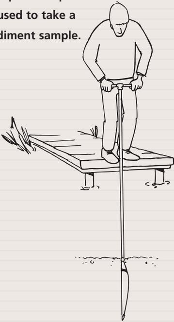
After pre-drilling with the Edelman auger a sample is taken of the wet peat with the peat sampler.
