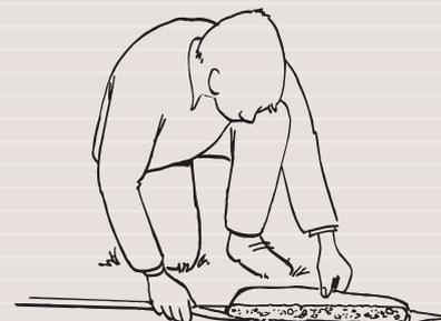
The Vrijwit auger is used to take a sample from the bottom of a ditch.
